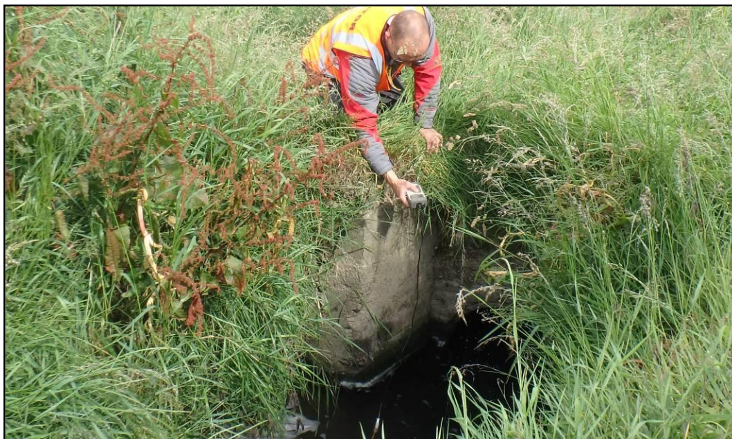
Plate 12 Reading Conductivity of the discharge to the River Nanny.
