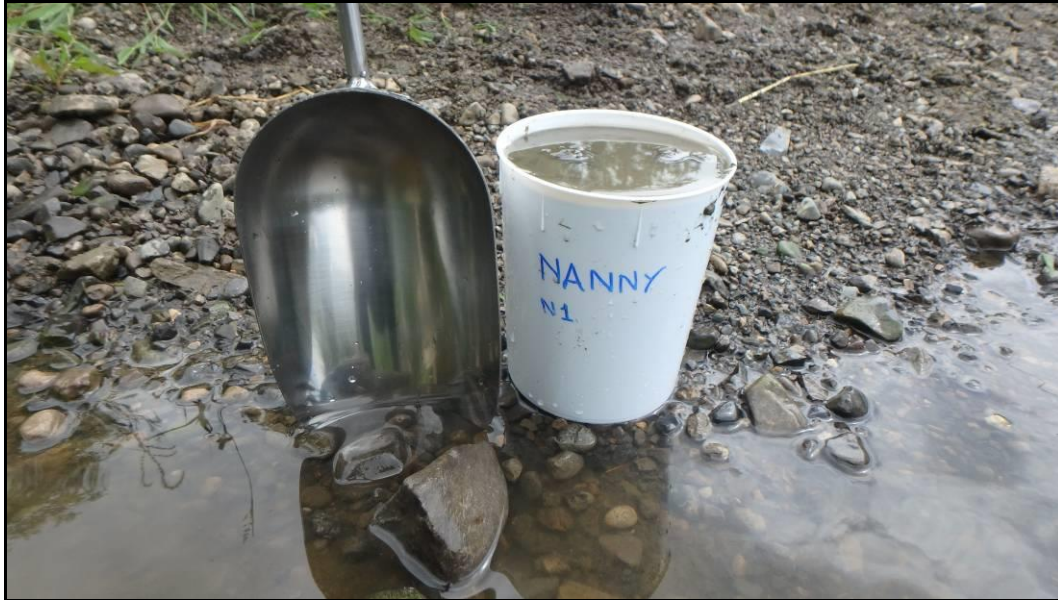
Plate 11 Particle size distribution sample from Site N1 showing the trowel used to obtain the substrate samples.
